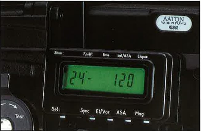
A back-lighted full-function LCD display monitors all camera operations: Sync speeds, x-tal controlled wild speeds, ISO selection, battery voltage, magazine remaining footage, last take elapsed footage, time code readout.
